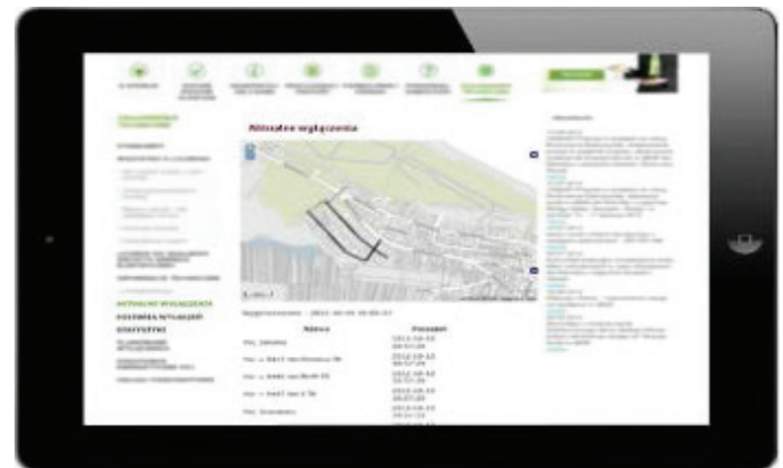
Fig. 3. Web portal with online in-grid presentation of effects of the outages currently registered in Syndis RV's OMS module
