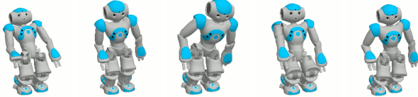
Fig. 4. Examples of valid goal configurations for a given pose of the robot’s right hand. The feet of the robot remain fixed, and the 5D goal pose for the hand is identical in all configurations. In this case, the left arm was set to a safe configuration adjacent to the robot’s body.
