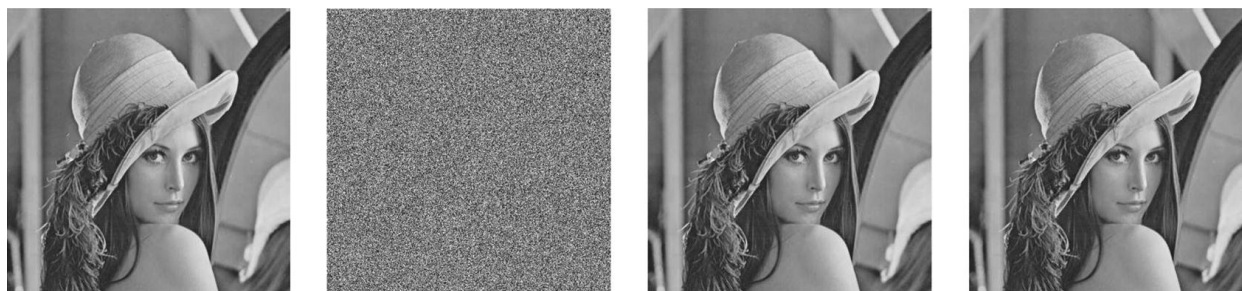
(a) Original image, (b) encrypted image, (c) decrypted image containing messages (embedding rate 0.1 bpp), (d) recovery version.
