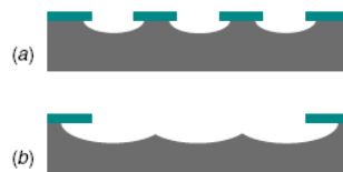
Figure 2: Under-etching phenomenon during isotropic wet etching
