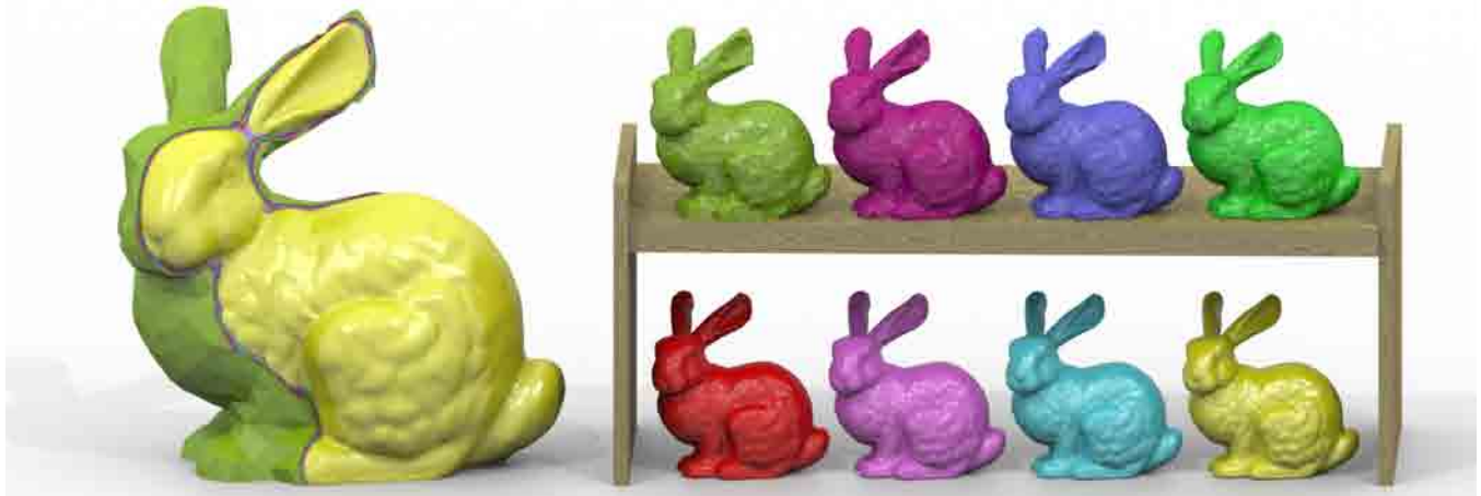
Figure 1: Given an input shape (yellow on bottom right), our method constructs nested cages: each subsequent mesh is coarser than the last and fully encloses it without intersections. A slice through all layers (left), shows a tightly encaged Bunny.
