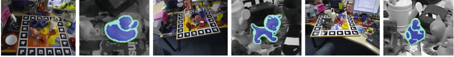
Fig. 3. Sample results from the experiments, for the ‘duck’, ‘cat’, and ‘ape’ sequences (left to right). For each result, shown is the RGB image on the left and a zoomed-in visualization of the estimated pose to its right (Color figure online).
