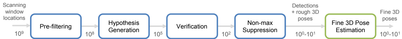
Fig. 2. Evaluation cascade of the proposed method. Note the typical numbers of detection candidates advancing through individual stages (for a template size 108 \times 108 px, a VGA input image and a scale space with four larger and four smaller scales with a scaling factor 1.2). A detection candidate is a triplet consisting of a template identifier (object and its orientation), a sliding window scale and a sliding window location.
