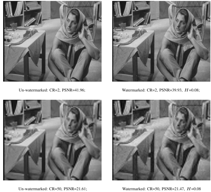
Fig. 2. Application example where distortion due to watermark embedding is adaptively negated at various JPEG2000 compression ratio (CR) without compromising robustness. H stands for Hamming Distance ( H \in 0..1 ), a commonly used metric of watermarking robustness. Lower value of H ensures higher robustness.
