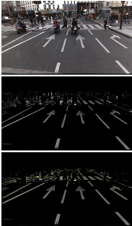
Fig. 7. From top to bottom : original image ; road marking extraction using 43 rd PLT ; road marking extraction using 43 rd PLT (in gray level) and edge information (in yellow).
