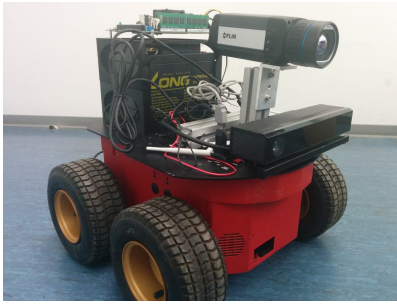
Figure 5: Pioneer 2 mobile robot equipped with a Microsoft Kinect v2 depth-sensing camera and a FLIR A655sc thermal camera.
