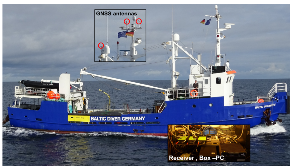
Figure 4. BALTIC TAUCHER II with the mounting of the antennas.
