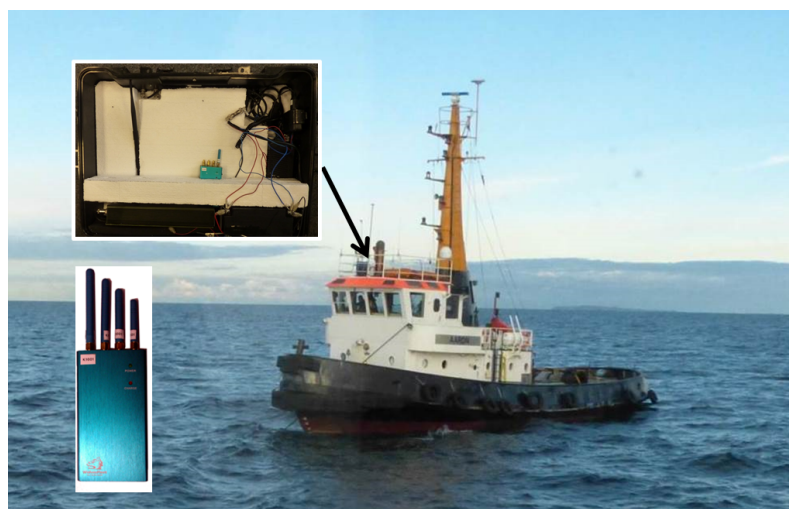
Figure 2. AARON with the jammer mounted on the monkey deck.
