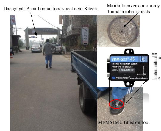
Figure 10. Urban canyon test environment; Daengi-gil, a food-street near Kitech. The IMU sensor is fitted on top of the left foot. In the upper right corner, a large metallic manhole cover, found in many urban streets, along with other large metallic objects are shown.
