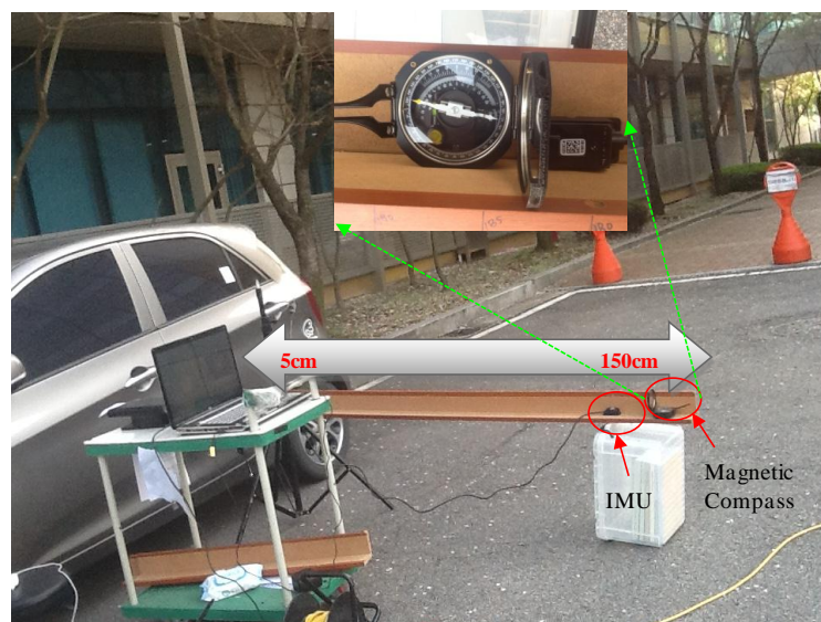
Figure 21. Moving IMU in an exact straight line, by sliding the sensor on a straight wooden support. In close-up is shown a very precise magnetic compass for reference heading.
