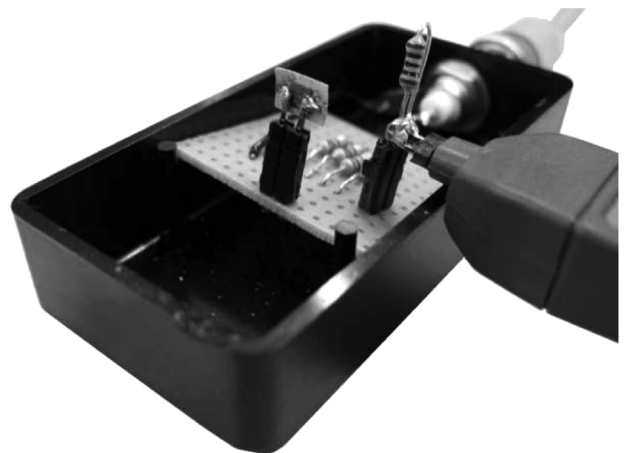
Figure 1 Setup for power-consumption measurements on a passive RFID tag
