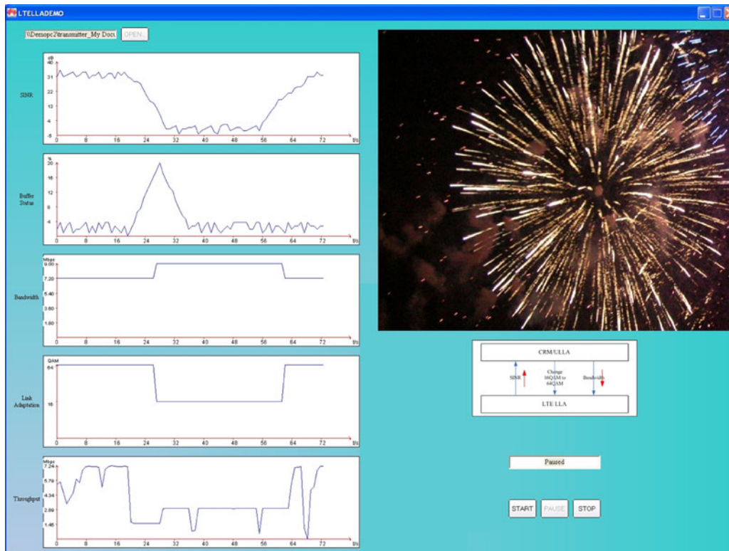
Fig. 13 Radio condition has improved and CRM increases modulation order and decreases bandwidth to ensure efficient use of radio resource
