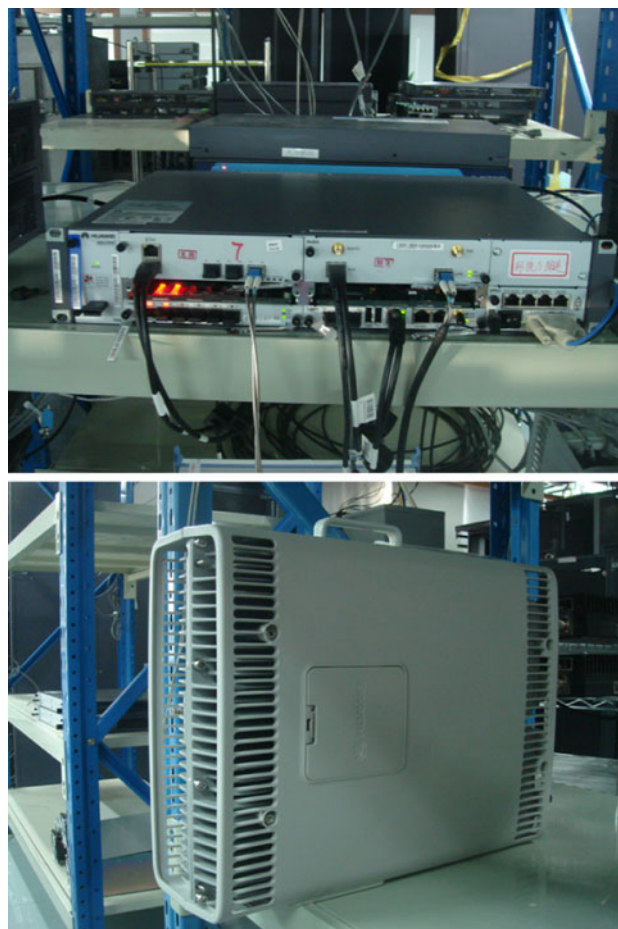
Fig. 3 LTE prototype equipment. Baseband unit (top), RF unit (bottom)
