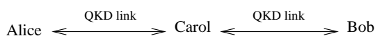
Figure 3: QKD bridge: Alice and Bob are out of the QKD range; they want to use Carol as a bridge to communicate securely the session key.
