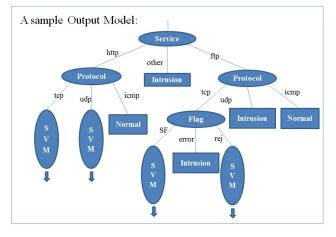
Figure 4: A sample model for anomaly detection
