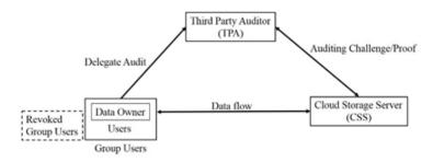
Figure 1: Public auditing with shared data in cloud data storage architecture **Security attack evaluation.** We list some common attack model and they can analyze whether public au-
