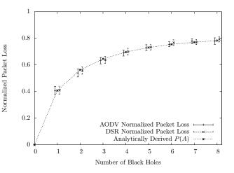
Figure 3: Normalized packet loss due to Black Hole attack for the 4x4 grid network
