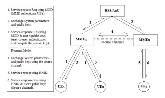
Figure 2: The proposed LTE-AKA handshaking process
