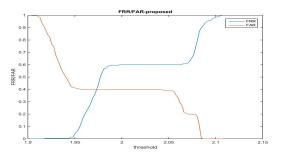
Figure 10: Performance of FAR and FRR for the Re-login authentication using MPCA with GSO
