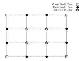
Figure 2: 4x4 Wireless grid topology with labeled source node classes
