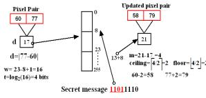
Figure 1: Data embedding through PVD with example
