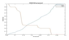
Figure 6: Performance of FAR and FRR for the continuous authentication using MPCA with GSO
