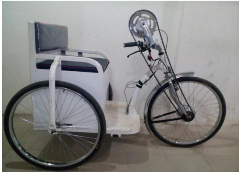
Fig 1.6: Existing Electrically Assisted Wheelchair with Torque Sensor
