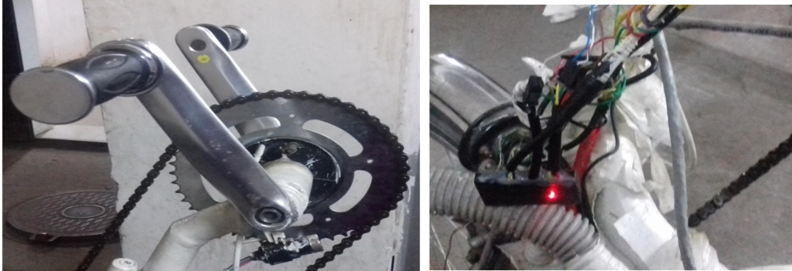
Fig 4.3: The torque-sensor pedal and module attached to the wheelchair
