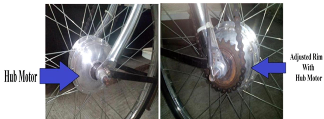
Fig 2.4: Hub Motor & the Adjusted Rim
