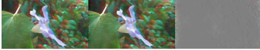
Figure 17: A snapshot of the original stereoscopic color video and the reconstructed stereoscopic color video. From left to right are respectively, the original video, reconstructed color video and the error. The 3D effects can be visualized by wearing red-cyan 3D glasses.
