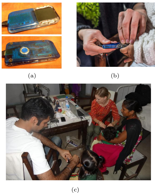
Figure 1: Fingerprint capture of infants. (a) The compact ( 7\text{cm} \times 3\text{cm} \times 7.5\text{ mm} ) and high-resolution (1,270 ppi) custom fingerprint reader, (b) fingerprint capture of an infant using the reader, and (c) fingerprint capture at two data collection stations in Dr. Bhatnagar’s clinic in Saran Ashram Hospital, Agra, India.
