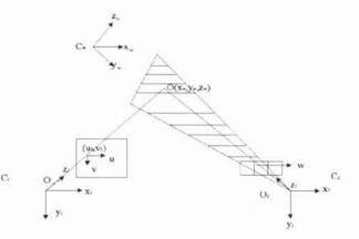
Figure 1: Determination of depth from a structured light.
