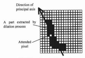
Fig.5. Detection of stroke direction
