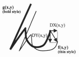
Fig.2. Correspondence estimation (definition of displacement amount DX, DY).
