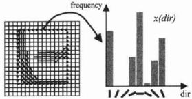
Fig.6. Drawing histogram x(dir) based on frequencies of stroke directions.
