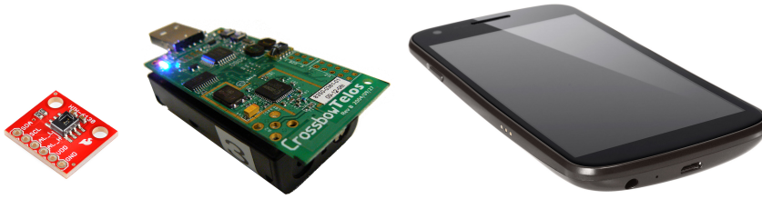
Figure 2.2: Examples of physical sensors: a humidity sensor (courtesy of Sparkfun.com), a TelosB sensor node, and a Galaxy Nexus Android Smartphone.
